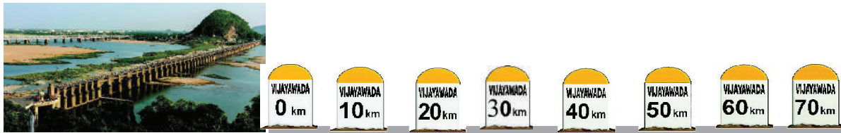
Fig. 5.13: Positions of kilometre stones with respect to Vijayawada as a reference point
