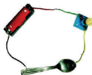
Fig. 3.18: (a) Conduction tester (b) Using the conduction tester for testing a material
