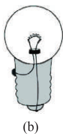
Fig. 3.4: (a) A small incandescent lamp used in a torch (b) its simplified drawing showing the connection of wires to the terminals
