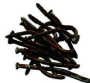
Fig. 5.4: Rusted iron nails
