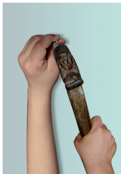
Fig. 2.7 : A nail is fixed in the wall due to friction
