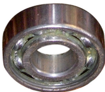
Fig. 2.16 : Ball bearings reduce friction
