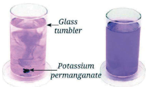
Fig. 3.13: (a) Streaks of pink colour spreading out; (b) Uniform pink colour in glass tumbler
