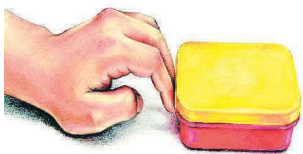
Fig. 2.5: Friction acts between two surfaces and opposes the motion of the object
